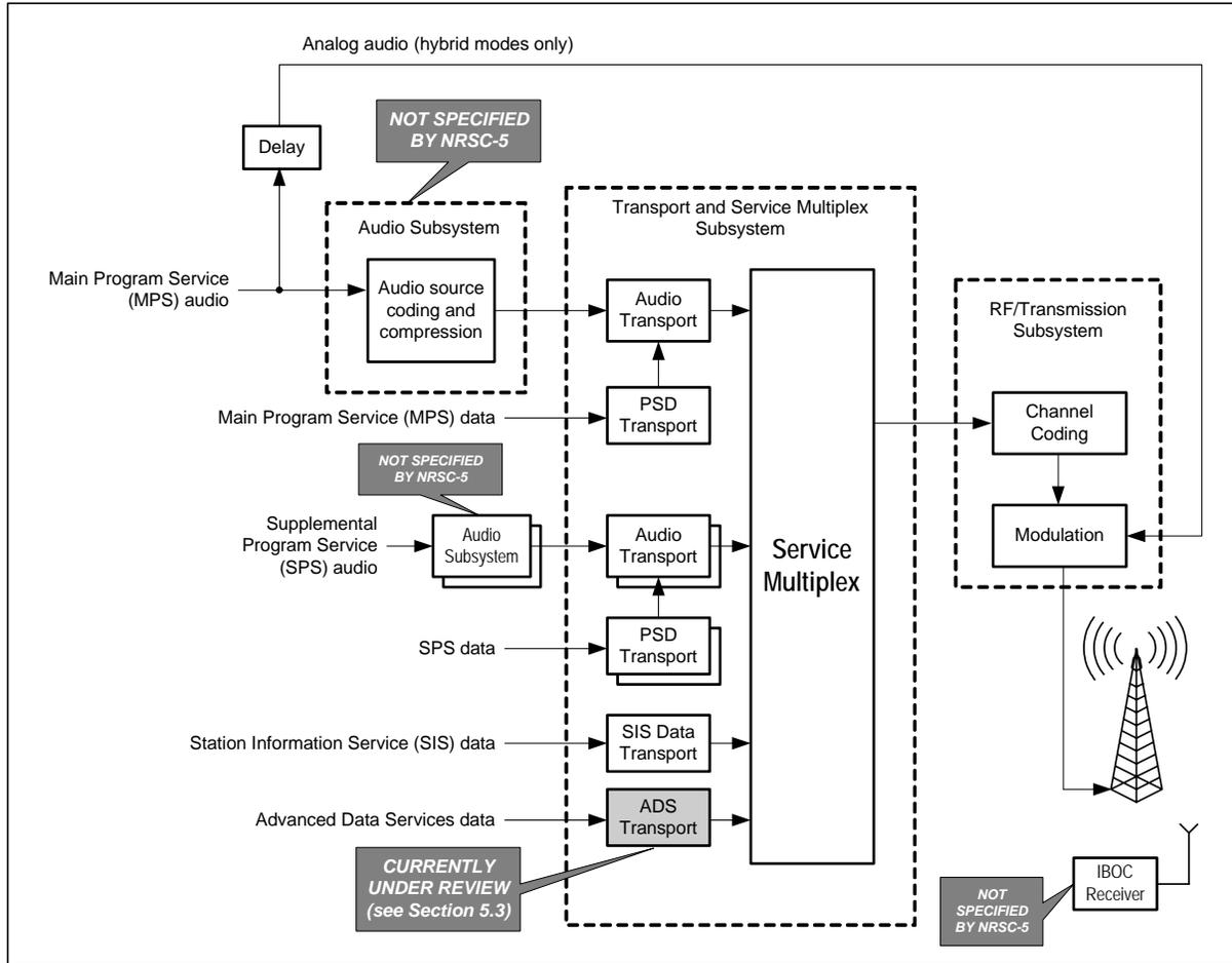
Figure 1: Overview of IBOC digital radio system
