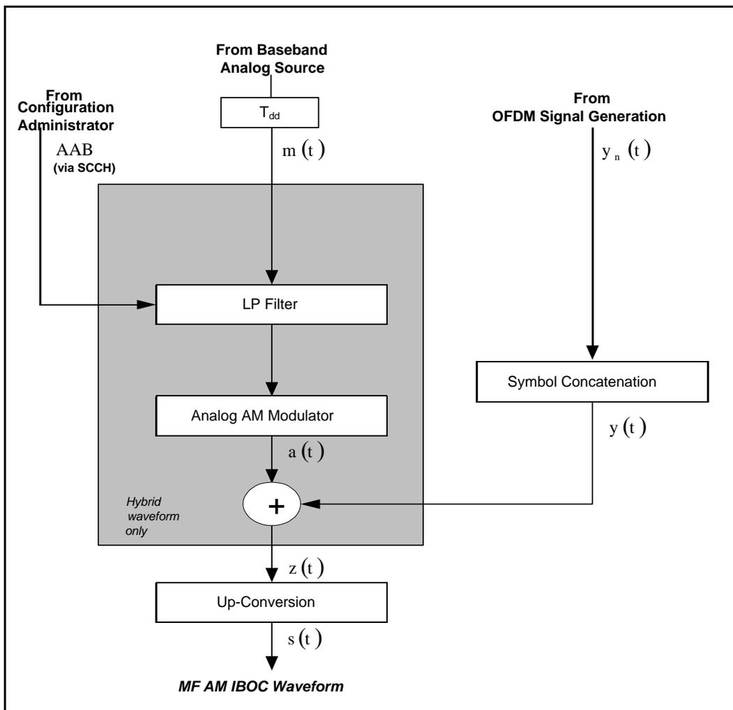
Figure 8: Hybrid/extended hybrid transmission subsystem functional block diagram
