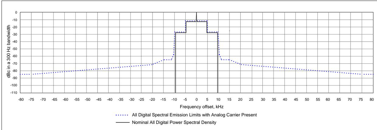
Figure 11. NRSC-5 AM all-digital waveform spectral emissions limits
