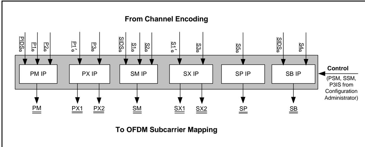
Figure 15: Interleaving conceptual block diagram
