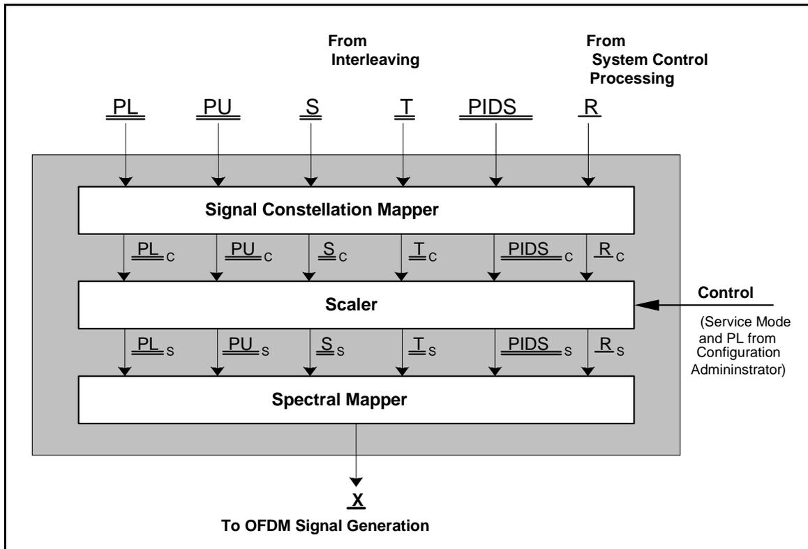
Figure 7: OFDM subcarrier mapping conceptual block diagram
