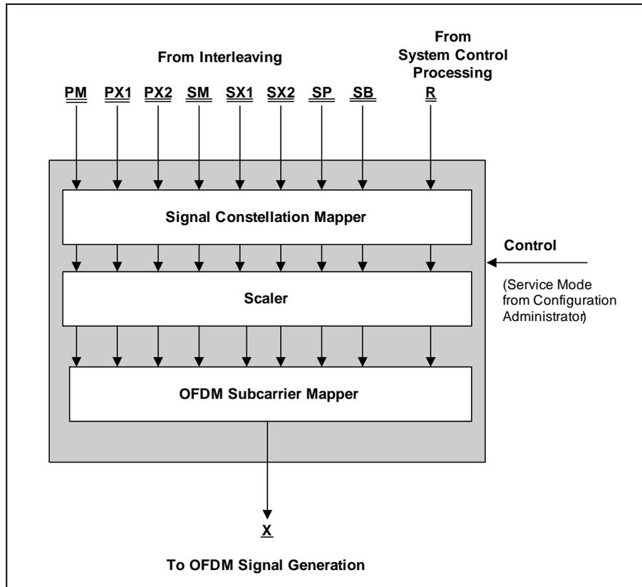
Figure 17: OFDM subcarrier mapping conceptual block diagram
