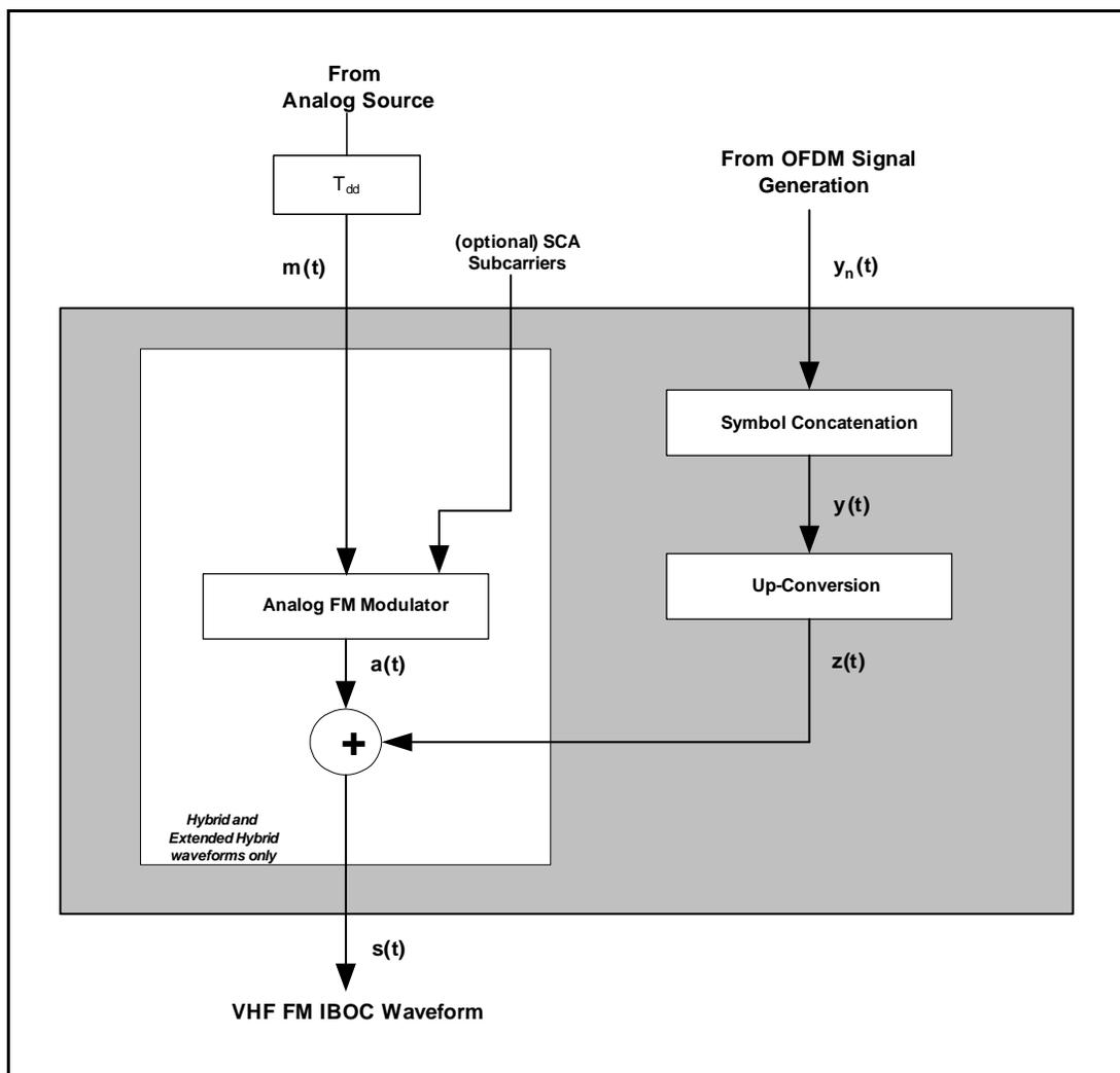
Figure 18: Hybrid/extended hybrid transmission subsystem functional block diagram
