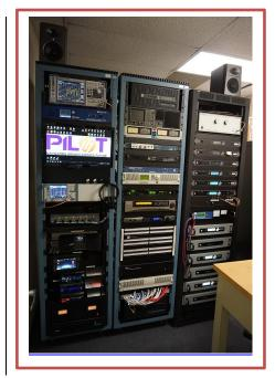
The existing test bed includes a transmitter rack, a receiver rack, and an audio rack. All racks incorporate grounding bars;
